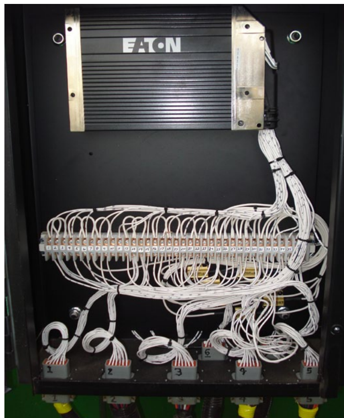
Four Eaton EFX programmable controllers are equipped on each AFE potato harvester.
